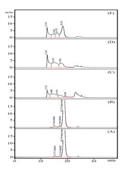
Fig. 3. The results of SE-HPLC: (A) Standard samples of IFN β-1a, (B) low pH treated IFN β-1a (C) 50 kGy Irradiated IFN β-1a, (D) 25 kGy Irradiated IFN β-1a, (E) 10 kGy Irradiated IFN β-1a.
