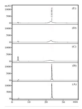
Fig. 2. The results of RP-HPLC: (A) Standard samples of IFN β-1a, (B) Low pH treated IFN β-1a, (C) 50 kGy Irradiated IFN β-1a, (D) 25 kGy Irradiated IFN β-1a, (E) 10 kGy Irradiated IFN β-
