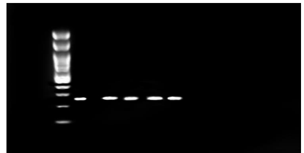
Fig. 2. The 274bp band shows a positive Nested PCR response against the ladder.
