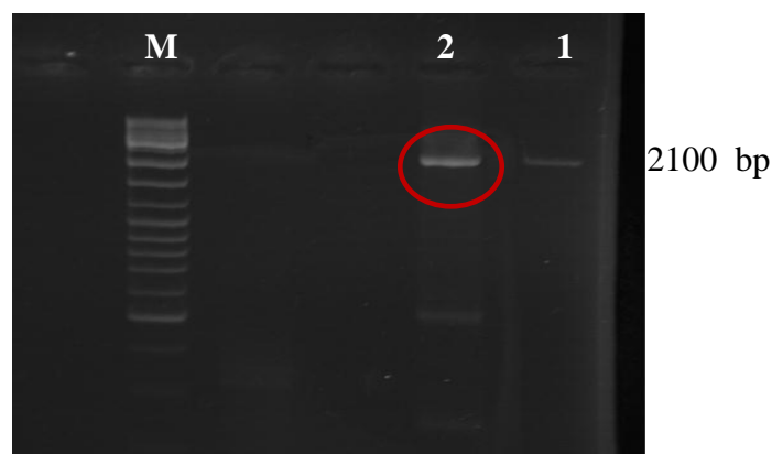
Fig. 4. RT-PCR analysis result (lane 2) was compared with PCR product (lane 1) and DNA ladder (lane M).
