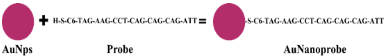
Fig 1. Schematic for probe attachment on gold nanoparticles surface by chemical interaction between thiol group and Au atoms.
