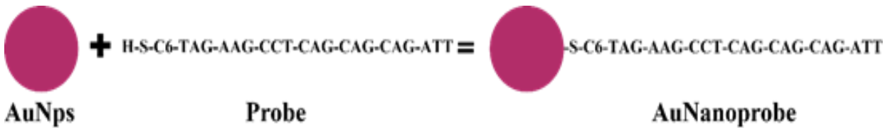
Fig 1. Schematic for probe attachment on gold nanoparticles surface by chemical interaction between thiol group and Au atoms.
