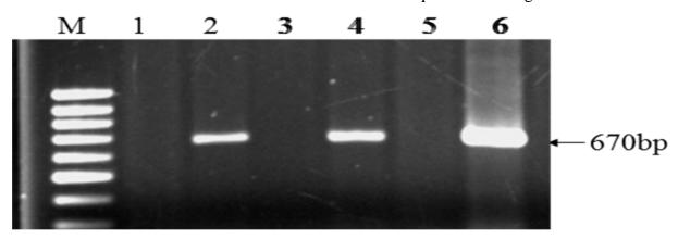
**Fig. 1.** PCR Detection of TYLCV-Ir2 specific 670bp band by using TYLCV-F and TYLCV-R: M) Marker (GenRuler<sup>TM</sup> 100bp DNA Ladder, Fermentase) Healthy plant 2) Tomato infected by *Bemisia tabaci* 3) nonviruliferous *Bemisia tabaci* 4) viruliferous *Bemisia tabaci* 5) Cauliflower, host of *Bemisia tabaci* 6) tomato plants infected in field (original source, Bandar-Abbas).
